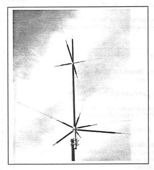
Although multi-band vertical HF antennas have limited band-width, the HVU-8 offers a good alternative for those seeking a compact/apartment antenna. The HVU-8 has surprising performance (if limited band-width) even on the 80M band
