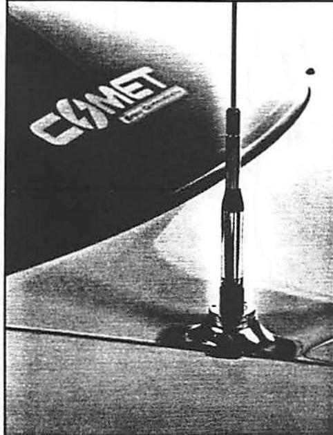
If stainless steel is your mount of choice, the GR-5M is pictured with an "SB" style antenna mounted. It's rounded for a more sleek appearance and uses all stainless steel hardware. Comet's deluxe cable assembly is included; total length is 16'4". Two offset washers adjust the antenna to vertical, and a soft rubber pad protects the vehicle paint. This mount will hold even Comet's biggest antennas.
