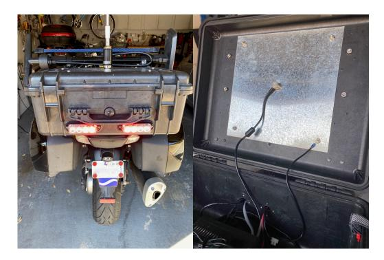
The Icom Radio and SR-10 is installed in a Pelican 1550 Weatherproof Case. On the inside top of the Box, I installed a "ground plane", even if the antenna (a Comet HP32-FHN) doesn't require it.
