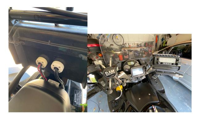
I used two Blue Sea Systems CableClam 0.68" as pass-through to get the wires out of the box. The RAM X-Grip Mount is for my iPhone.
