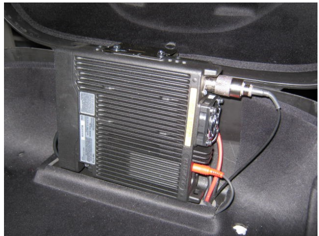
Fig.1. Radio Mounted inside front of Trunk
