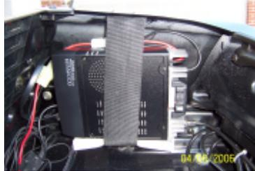
The radio is mounted on the right side of the trunk. I used a 2" wide strip of Velcro fastened at the top and bottom to hold my radio in. I already had a piece of 1/2" thick foam that I cushioned the radio with ( be careful to allow for ventilation).
