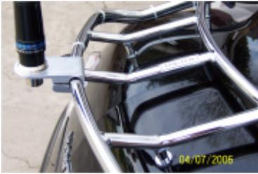
The antenna was mounted in the back and center of the trunk rack, which required modifying the mounting bracket to allow the center rack bar to come out of the center of the bracket. I put it in my vice and drilled a 1/2" hole in the bracket with the bracket closed tight. After drilling the hole I still had to grind a bevel on the edge of the hole to allow for welds on the rack.
