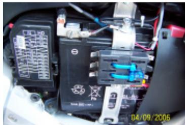
Power is easy. Be sure to power your FRSet 4 from the bike auxiliary circuit so it will turn off with the bike power. I wired it to my new fuse block and found I had no way to turn it off. It was an easy fix to move it over to the bikes accessory
