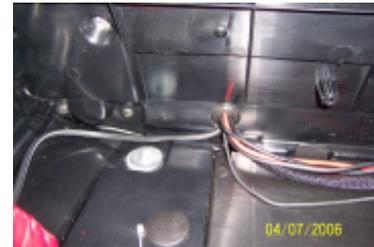
A 3/4" hole was drilled in the left side of the trunk for the wires. I added a rubber grommet to help protect the wires. Be sure to remove the seat first and drill from the seat side so you wont puncture the seat.
