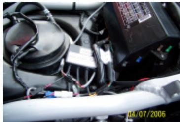
I found all the connection points per the instructions and located the FRSet 4 under the seat as you see it in the picture. Due to all the fixed lengths on the cables that is where it wanted to be mounted. Be sure to set the dipswitches according to the instructions and test the audio volume before you remount the seat.
